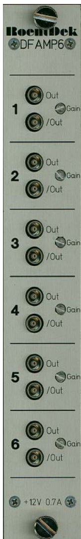
Figure 3.7b: DFAMP6 front panel with signal outputs and gain potentiometers
