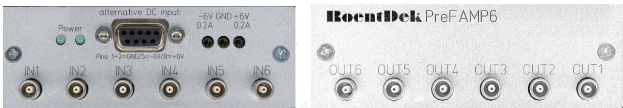
Figure 3.10a: Rear panel of PreFAMP6 (left) with signal inputs and DC power input via 9-pin sub-D connector or sockets for 2 mm pins (+12 V version provides a power output for daisy-chaining instead of the 2 mm pin sockets). Right: front panel of PreFAMP6 with signal outputs.
