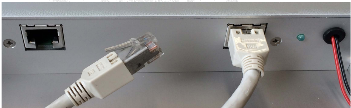
Figure 3.8a: Rear view of a FAMP6 with power connector to NIM bin and signal inputs. Above: LEMO sockets, below: differential inputs via special CAT6 connector
